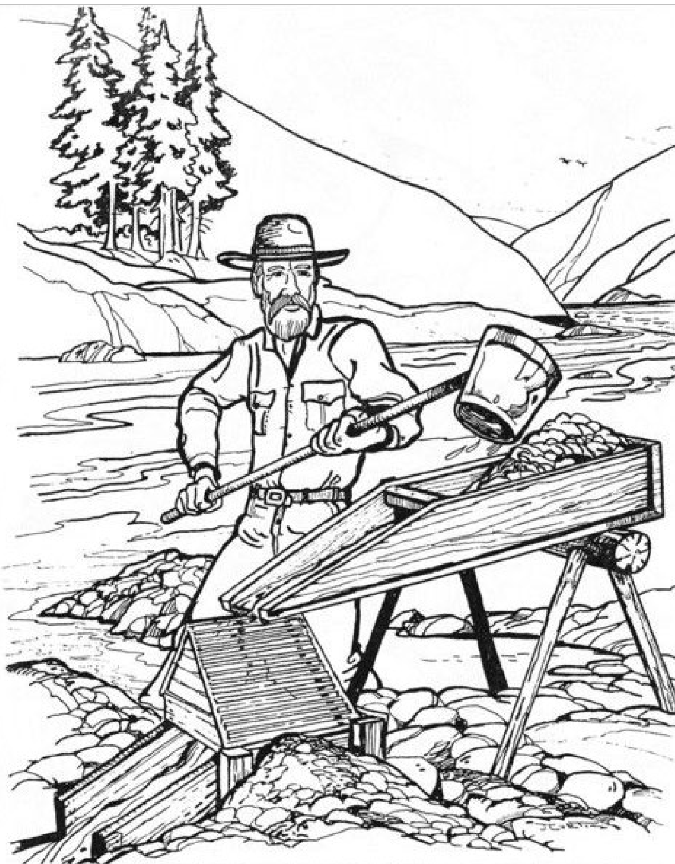
Miners tested gravel on the river's banks. Gold was found. This miner is washing river gravel with a Long Tom.
